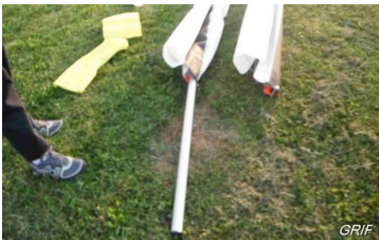
Match the correct leading edge tube (red is the port or left side when viewed from behind the wing).
