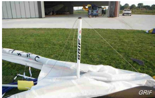
Check that the luff lines and cables are in good condition and aren't twisted or kinked.
