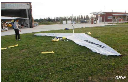
Spread the wings slowly in stages. Stop if any resistance is felt.
