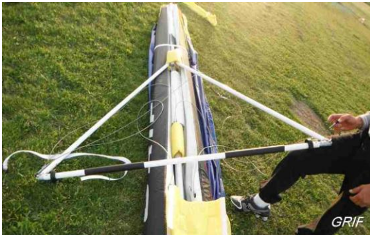
Assemble the A-frame without tangling any cables.
