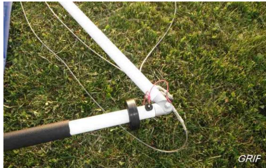
Insert the push-pin from the front of the A-frame and secure.
