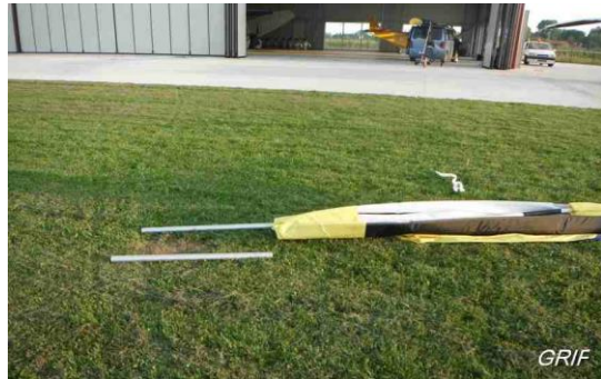
If the wing has been short-packed, retrieve the outer leading edges.
