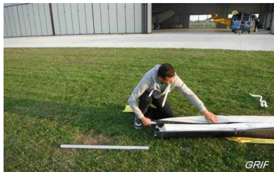
Insert the outer leading edges in turn and ensure they are fully home. Check that the sprung pin is fully secure- preventing the outer leading edge from rotating.
