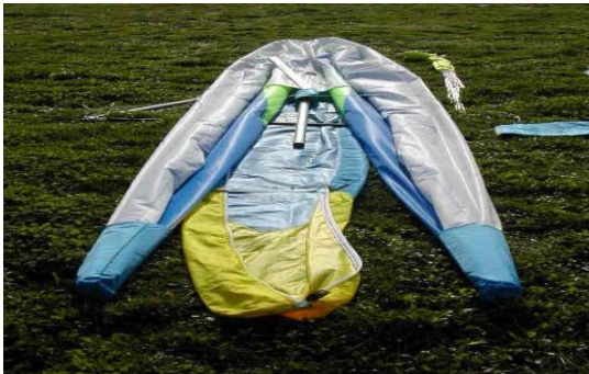
Roll the wing onto its front, laying the A-frame underneath the wing.
