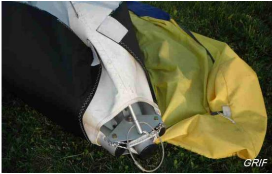
Insert the nose batten and locate over the foremast bolt in the noseplate.
