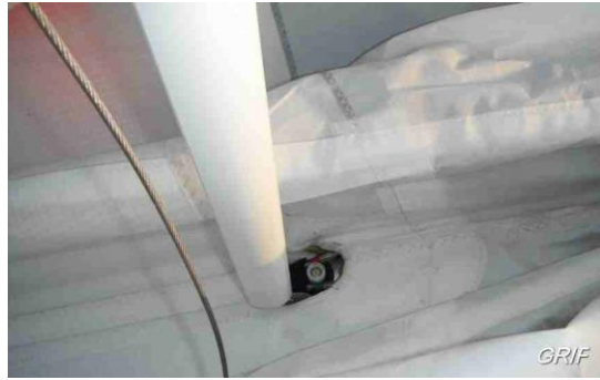
Check the pull-back cables aren't twisted and are free to move.
