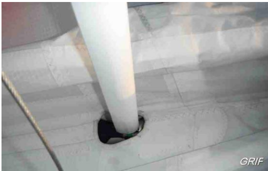
Position the kingpost fully home and ensure the pull-back cables are on either side of it (red to port).
